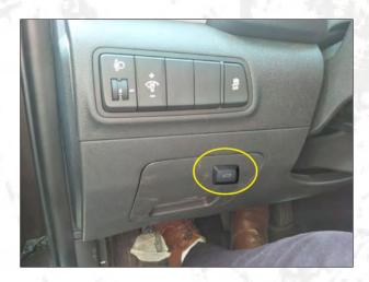
9.Remove the trim panel at the main driver's seat. Punch and install our front switch button.
