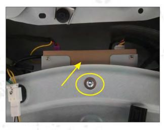
18.Install our central control box and fix it with our screws and gaskets.
