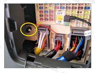
8. Find the ground screw on the left side of the main drive power and connect the ground wire.
