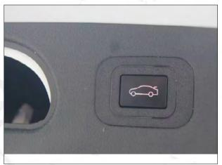
20.Install tailgate switch to position as shown in the picture.
