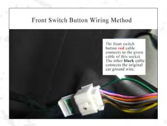
16. The cable thrown by the front swithc of the main drive's seat is connected to this socket at the tailgate.
