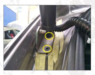
4.Remove the original car bracket. Install our left lower bracket and fix it with our screws.
