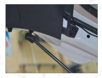
2.Reomve the snap rings and the original car brace rod, and then install our company's brace rod with the original car ball head.
