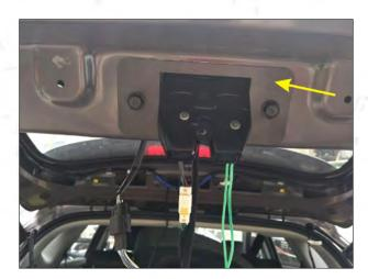
12.Our yellow central control cable is connected to the blue cable (The second hole in the first row from left to right).
