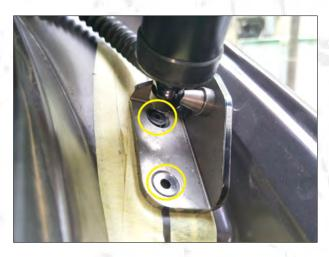
3.Remove the original vehicle bracket. Install the lower right bracket of our compay and fix it with our screws.
