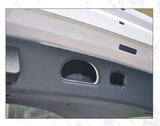
19.Remove the small cover of the lock cover and cut the plastic in the square of the cover with a knife.
