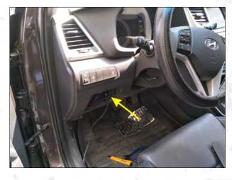
6.Remove the trim panel under the main drive and find the power supply.
