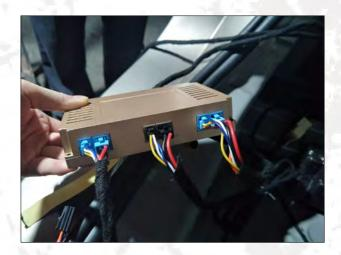
17. According to the color, insert the hall line, the power cable and the electric suction cable to the control box.
