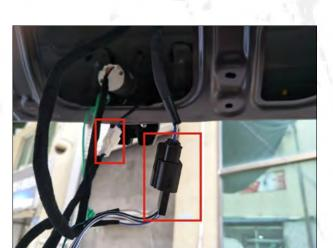
14.Unplug the three-way socket of the original car. Insert our three-way adapter socket and then connect the socket of the door lock to the socket of the three-way wiring harness.
