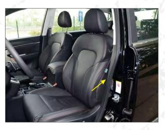
11.Remove the trim panel at the main driveing seat belt B-pillar and find the central control.
