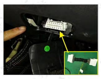
10. Find the original car OBD under the main driver's seat and insert the OBD adapter socket.
